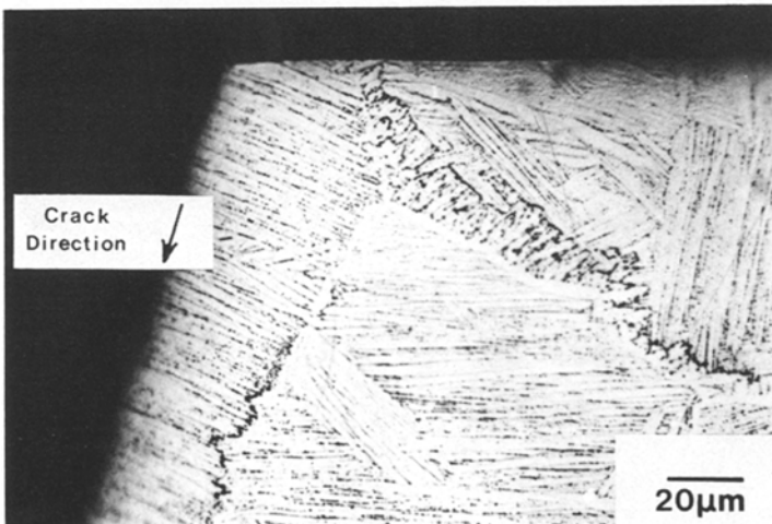
Figure 7 Fretting fatigue crack initiating and propagating across the boundaries of the \alpha -platelets. Tested at 400° C, low fatigue stress.
