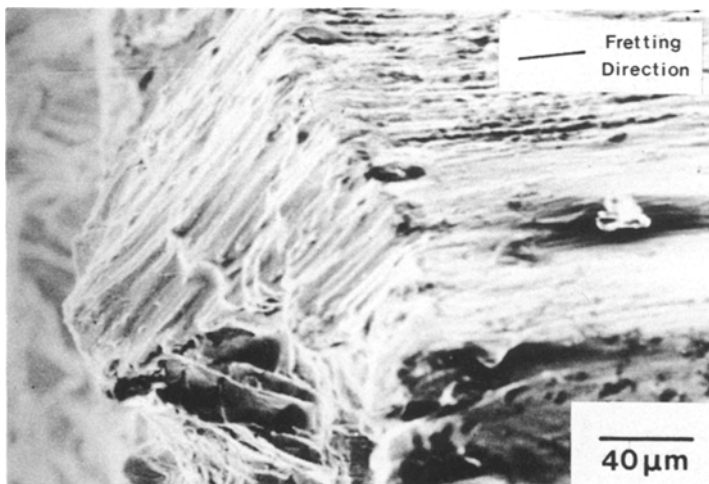
Figure 18 Fatigue crack initiation and growth at 45° to the surface of the specimen. Test temperature 600° C; high fatigue stress.
